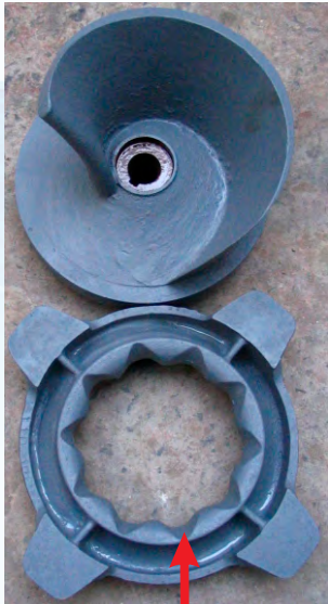
Macerating ( Cutting/ Shearing ) Inlet Bell Mouth edges
