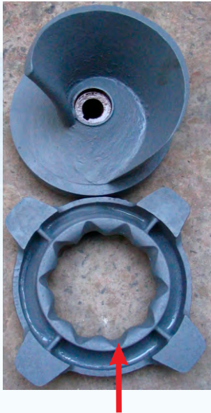
Macerating ( Cutting/ Shearing ) Inlet Bell Mouth edges
